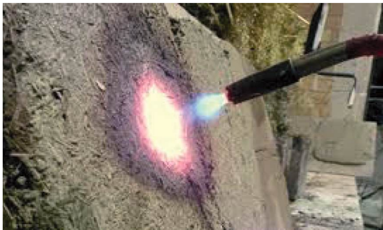
A naked flame on Hempcrete
