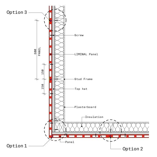
Liminal recommends control joints be located at the corners of the junction of the panels, that is set at 35mm back from the corner as detailed as Option 1. If this is not preferred, the control joint can be located at the first panel joint at 600mm Option 2, BUT the maximum spacing from a corner is 1200mm Option 3. On straight runs of walls, control joints must be installed every 6 metres
