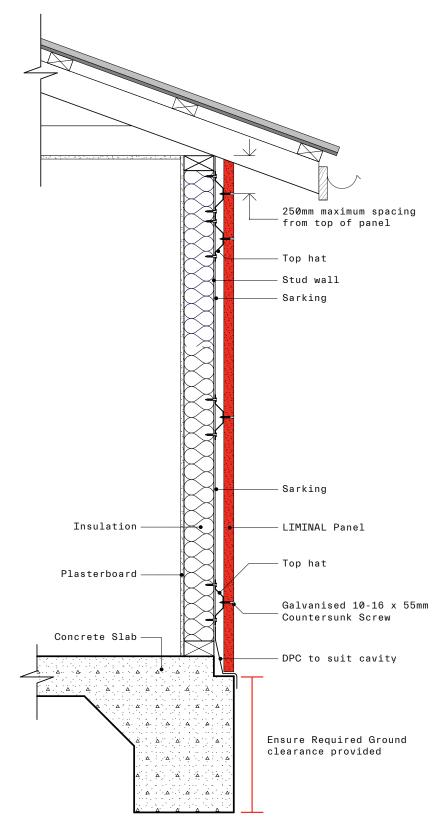
Note: Top hat spacing to be a maximum 250mm from the top and bottom of the panel.
