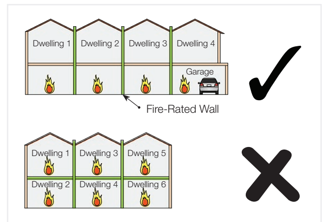
FIGURE 1 HARDIE™ SMART INTERTENANCY WALL SYSTEM TYPICAL APPLICATIONS
