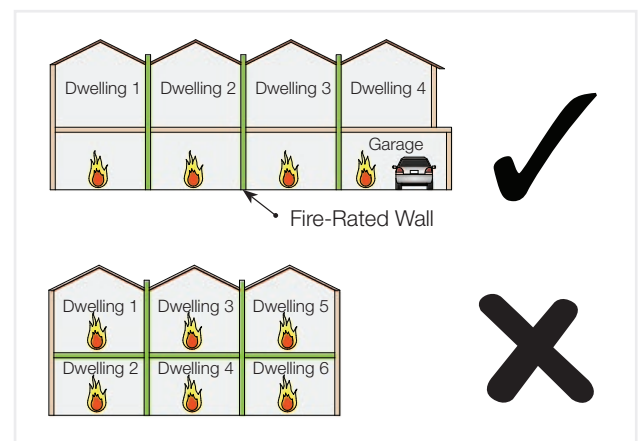
FIGURE 1 HARDIE™ SMART INTERTENANCY WALL SYSTEM TYPICAL APPLICATIONS
