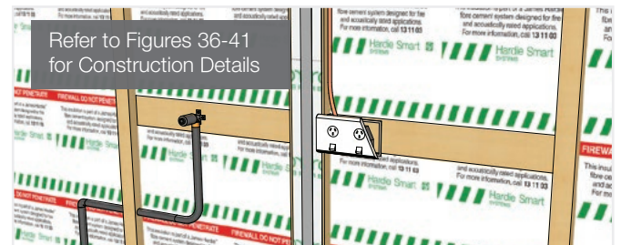
FIGURE 21 INSTALLATION OF SERVICES
