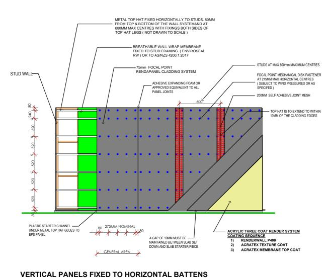
SCALE 1:50 - FIXING LAYOUTS FOR 75MM THICK PANELS
