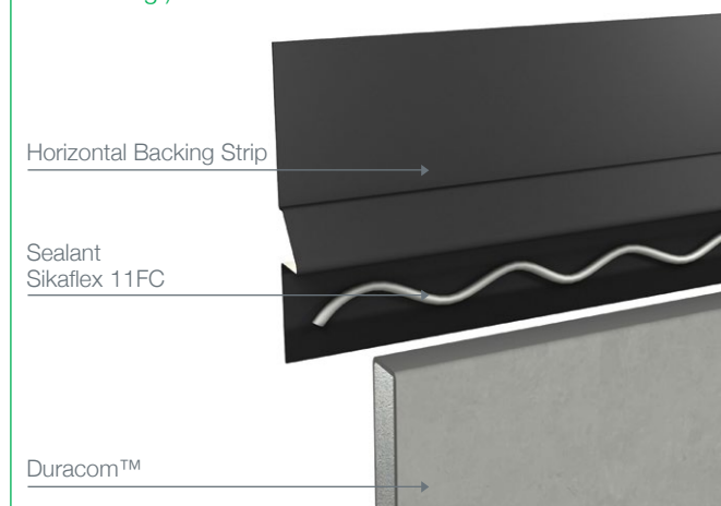
Figure 5 Sealant (Preferred Option for Optimal Adhesion and Sealing) - Front View
