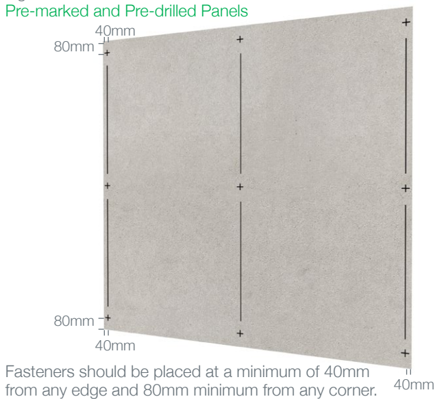
Figure 4 Pre-marked and Pre-drilled Panels
