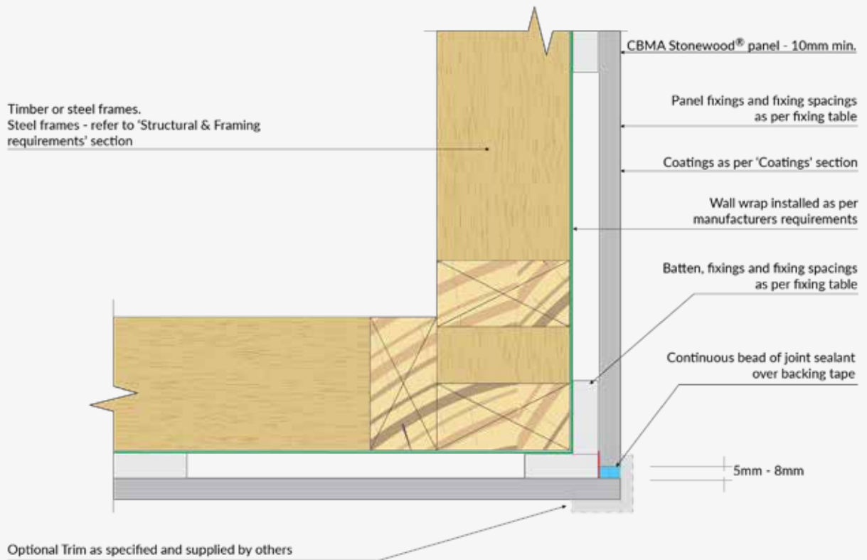
STONEWOOD® CAVITY FIX - TYPICAL EXTERNAL CORNER DETAIL DIAGRAM 13
